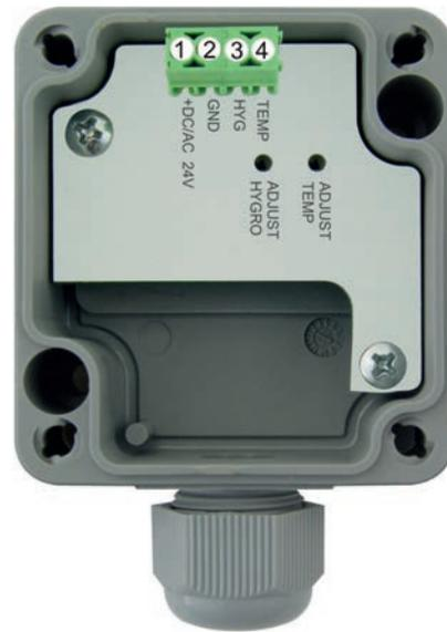
Temperature and humidity is always with reference to GND, operating voltage +DC/AC 24 V is common for both transmitters. The measurement of the output signal should be done with separate signal ground, in order to avoid measuring error due to voltage drop at the supply ground.
