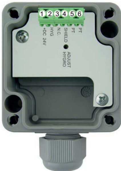
The shielding (SHIELD) is to be optionally covered. Connection through shielded lines is recommended.
