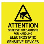
This sensor is sensitive to damage from ESD. Normal precautions as usually applied to CMOS devices are sufficient when handling the device. Touching the signal output pins has to be avoided at any time before soldering or plugging the device into a motherboard.
