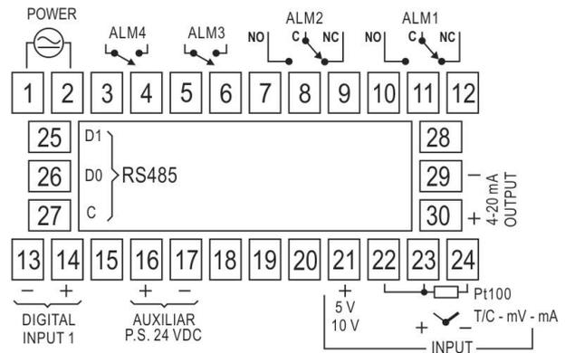
Fig. 1 – Back panel terminals
