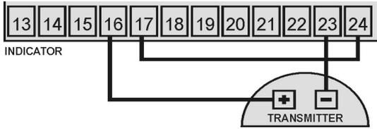
Fig. 9 – Two-wire transmitter with internal power supply
