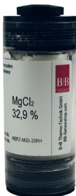
The module is supplied in calibrated condition. The accuracy at 23 °C is of the order of  $\pm 0.3$  °K and  $\pm 2\%$  RH. Under normal operating conditions, it is not necessary to again calibrate the module. The measuring accuracy of humidity measurement portion can be done by the end user with the salt reference cells available as special accessories. The checkup must be done in temperature stable environment.
